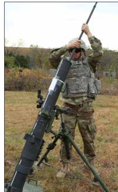
Barrel Cleaning: The barrel of a 120mm mortar system is cleaned by a Nebraska National Guard mortarman after firing a few rounds during a three-day, live-fire training.
